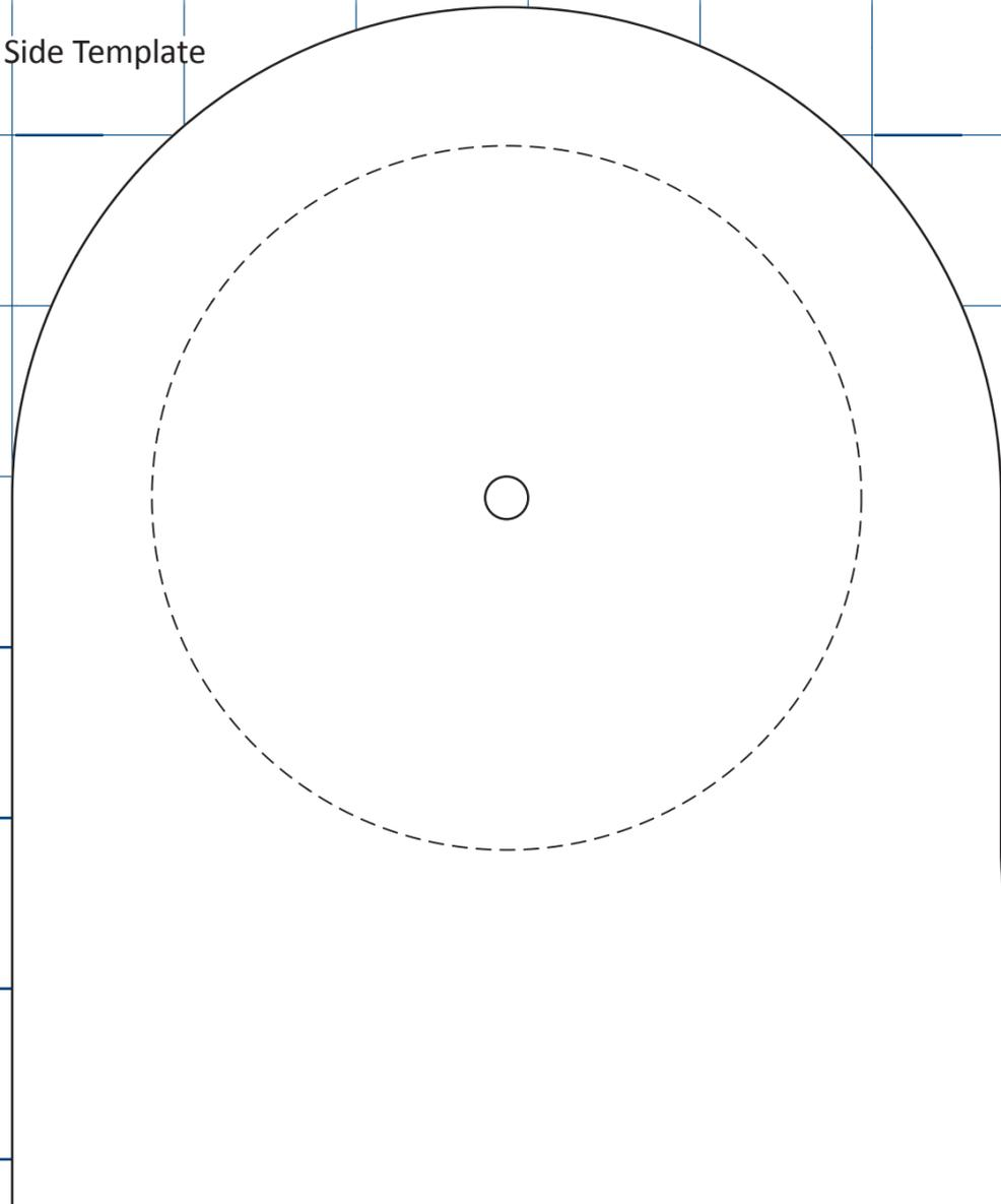
Note: For full-sized lathes, lengthen the sides to accommodate the maximum swing of your lathe while providing clearance for the dust collector pipe.
